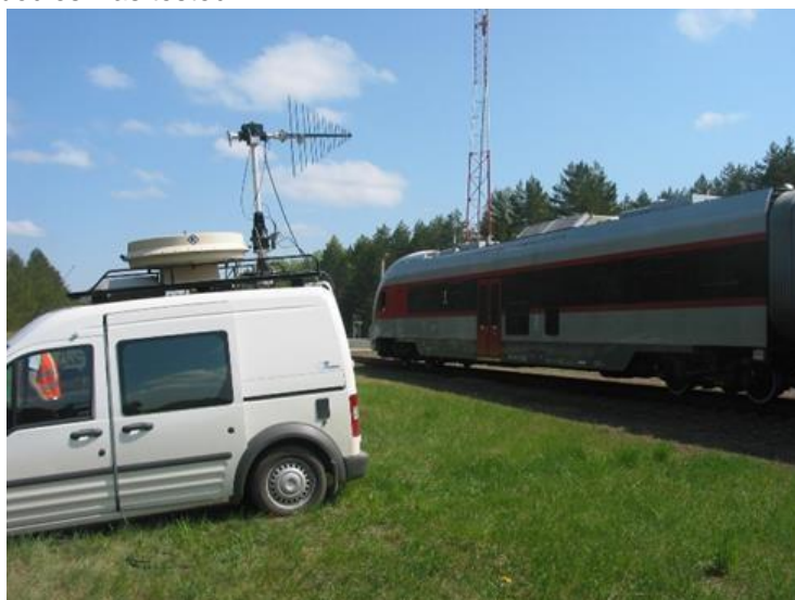
Fig. 23 RRT special-purpose vehicle parked at a track measures electromagnetic disturbance emissions of a running train.
