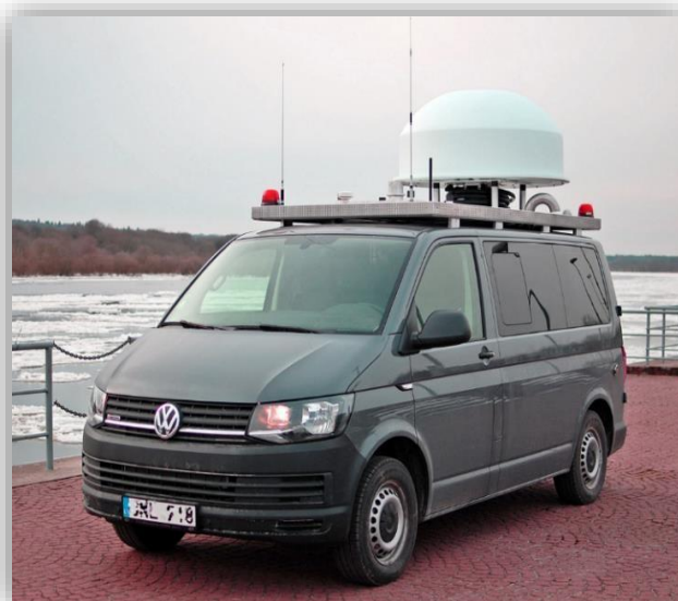
Fig. 32 Vehicle with a mobile spectrum monitoring
