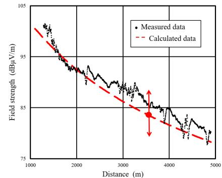
Fig. 4. The field strength level as a function of the distance from the transmitting antenna along a route which coincides with antenna's beam axis. is the measured radiated power  $P_m$ .
