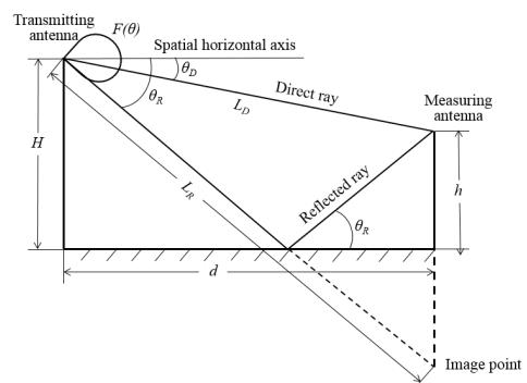
Fig. 2. Geometry of the two-ray ground reflected model.
