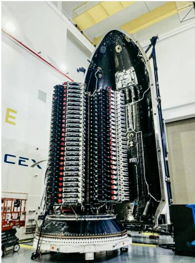
A stack of Starlink satellites awaiting encapsulation inside the payload fairing before a previous Falcon 9 launch. Credit: SpaceX
