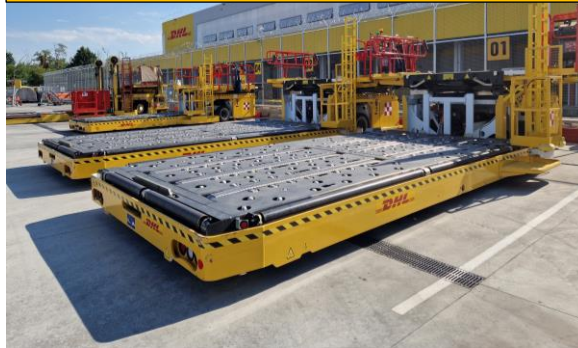
Malpensa Hub – TLD electric Highloaders (14 tons)
