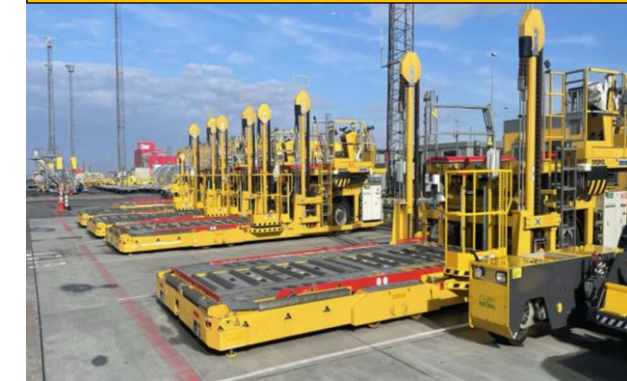
Copenhagen Hub – Electric Trepel Highloaders (14 Tons)
